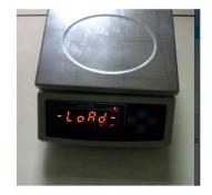
1000.0 means 1KG, you need to put 1kg weight on the plate. If it shows 2000.0, you need to put on 2kg weight on plate. Press [TARE] to confirm.
