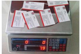
3. Press the quantity you had put on plate (here I need to press [6] ) and press [SAMPLE] key
